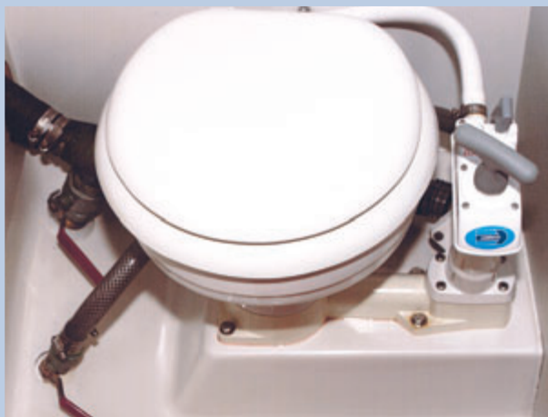
Give your head a thorough inspection and a good flush of seawater to clear the antifreeze.
